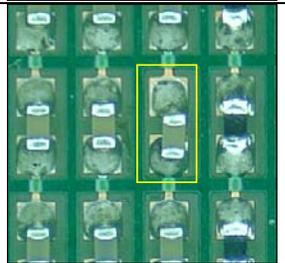
A micrograph showing a grid of chip components. A yellow box highlights a component in the second row from the top that is misaligned in its X-Y position.                                                                                     |
