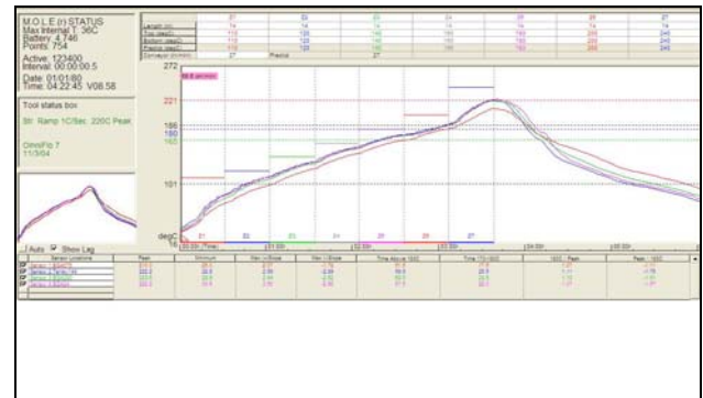
Figure 3. Ramp profile for Tin-Lead alloy. Ramp rate is 0.9 C/sec. Peak temperature is 210-220 C.
