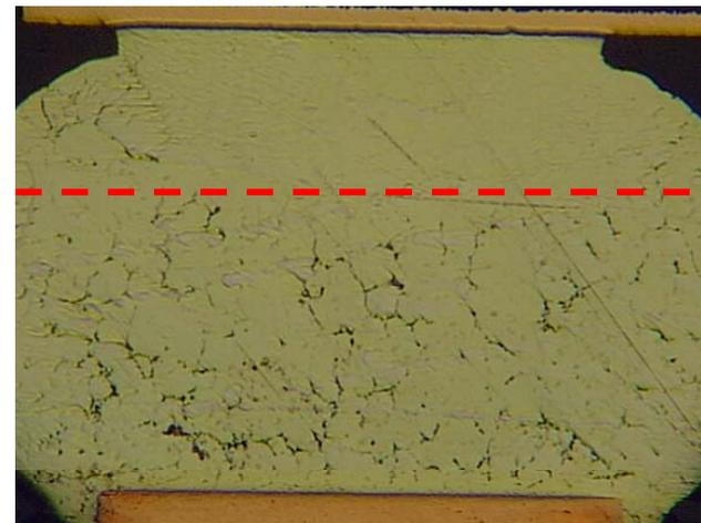
**Figure 6.** Cross-section of 1.27mm SBGA, SAC305 sphere with SnPb paste, reflowed with peak temperature of 215C and TAL of 60 seconds.<sup>3</sup>
