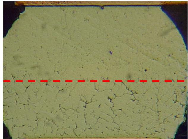
**Figure 5.** Cross-section of 1.27mm SBGA, SAC105 sphere with SnPb paste, reflowed with peak temperature of 215C and TAL of 60 seconds.
