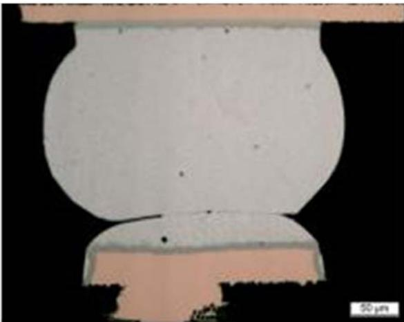
**Figure 1.** Low Silver BGA sphere with SAC305 solder. Notice the solder reflowed, but the sphere did not collapse.
