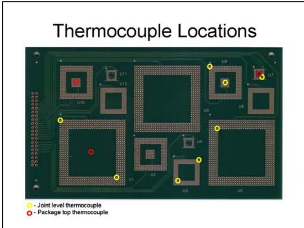
**Figure 4.** Thermocouple locations. The yellow circles indicate locations within solder joints; the red circles indicate locations on package bodies.
